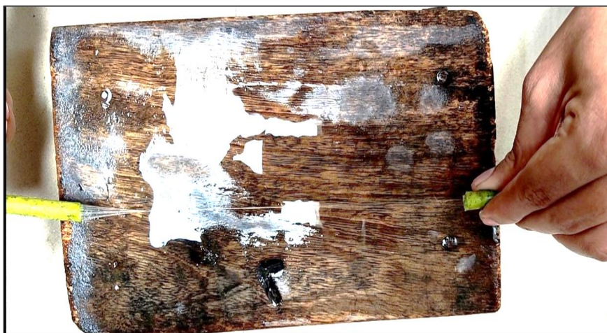
Figure 6. Extraction of Nelumbo stem fibres
